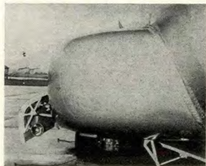
Hail and jets don't mix well. These photos show results of one such encounter between hail, C-141.
